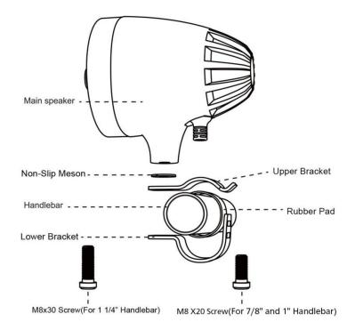
**Step 1:** Mount each speaker with its clamp to the handlebar of the motorcycle. *Note: Different size handlebar please insert different slot of the bracket as below.*
