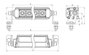
A - \frac{11.81" - 52.91" \quad C - 1.71" \quad D - 1.82" \quad E - 2.43" \quad F - 1.57" \quad G - 0.72" \quad \quad \quad 13.62" -
