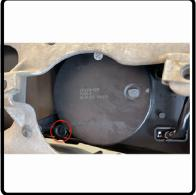
Remove the cap to access the adjustment set screw
