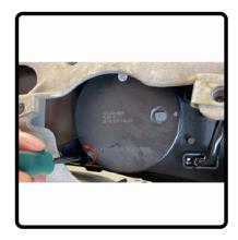
With the tool spin the set screw counter clock wise lower the low beam
