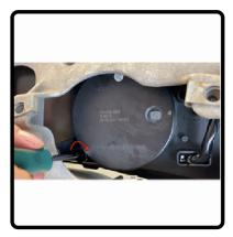
With the tool spin the set screw clock wise raise the low beam
