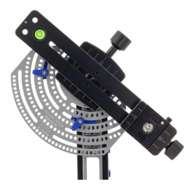
Point the camera to the upmost region of interest without touching the lower rotator. Engage the stopping plunger by lifting the lever. Loosening the end tab handle and slide the stopping tab against the vertical rail stop and tighten. This sets the upper limit and ensures camera and lens will not inadvertently touch the pano head during up and down rotation.
