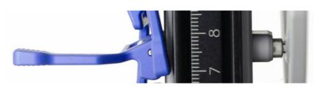
Stopping plunger in action. Front pin engaged.
