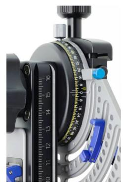
Rotate the index ring by 180 degrees. Align the 0 degree mark accurately and tighten the light blue screws to fix the index ring.
