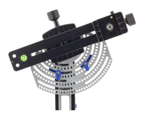
Point the camera to the lowest region of interest without touching the lower rotator. Engage the stopping plunger by lifting the lever. Loosening the end tab handle and slide the stopping tab against the vertical rail stop and tighten. This sets the lower limit and ensures camera and lens will not inadvertently touch the pano head during up and down rotation.
