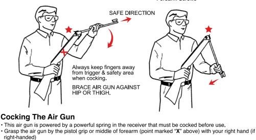
Avoid trigger and safety area when the breech of the gun is open. · With the unloaded air gun pointed upwards, apply a burst of firm pressure to the barrel as far forward as
