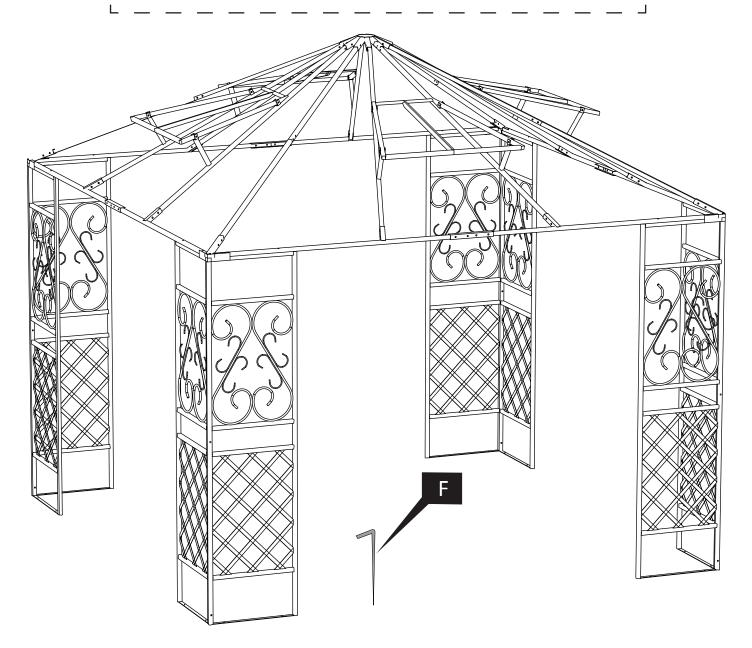
If the final location for your gazebo is a soft surface, you may secure it by driving the provided stakes (part F) through holes at the bottom of each gazebo leg panel (parts A and B)
