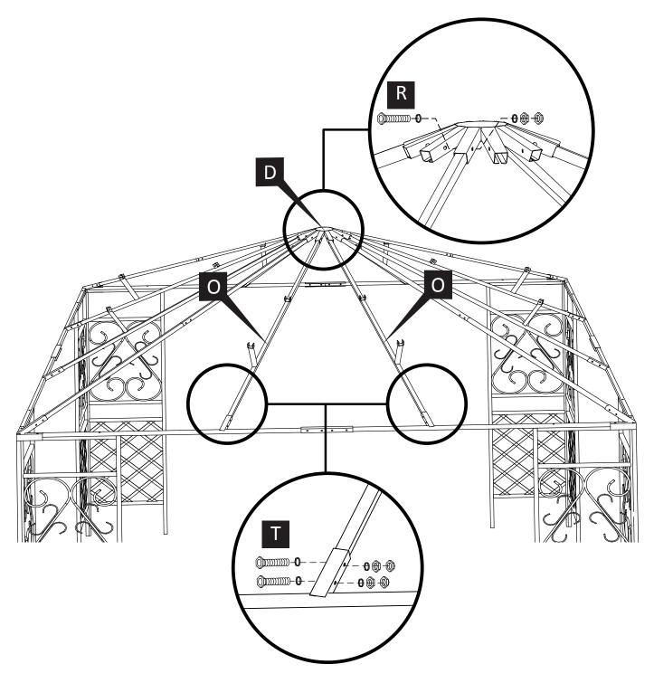
Attach the canopy vents to roof frame
