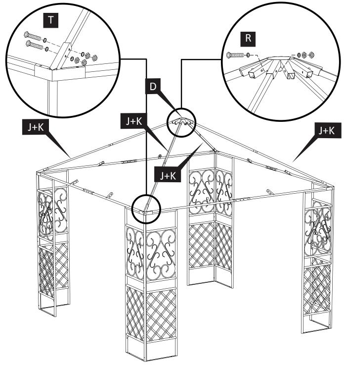
Attach the center support bars to the canopy frame [x 8]
