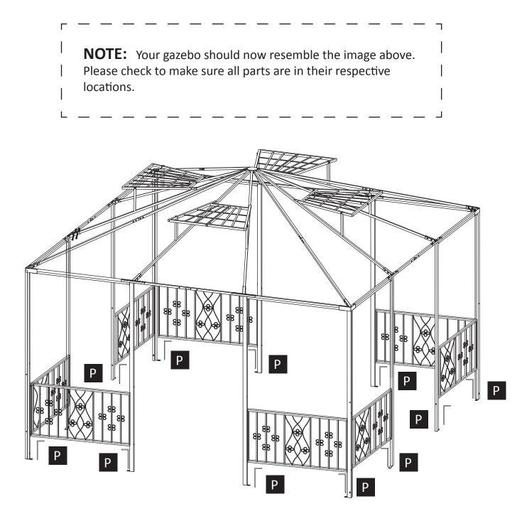
If the final location for your gazebo is a soft surface, you may secure it by driving the provided stakes through holes at the bottom of each frame column (A1, A2, A3).
