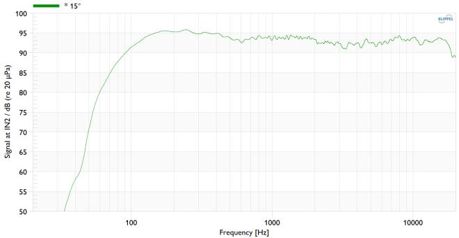
The SBS.1 frequency response and dispersion characteristics has been tuned and verified using Klippel™ software and an anechoic chamber.
