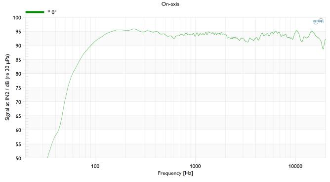
The SBS.1 frequency response and dispersion characteristics has been tuned and verified using Klippel<sup>TM</sup> software and an anechoic chamber.
