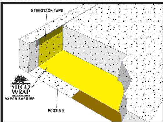
1. Stego Wrap can be installed over an aggregate, sand, or tamped earth base. It is not necessary to have a cushion layer or sand base, as Stego Wrap is tough enough to withstand rugged construction environments.
