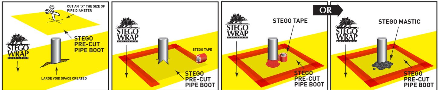
FIGURE 5: MULTIPLE PIPE PENETRATION SEALING
