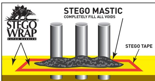
**MULTIPLE PIPE PENETRATION SEALING:**
