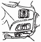
Press down starter switch button to use electric
