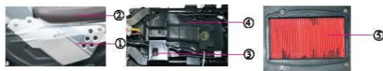
① Side cover ② Seat ③ Screw ④ Air cleaner cover ⑤ Air cleaner element
