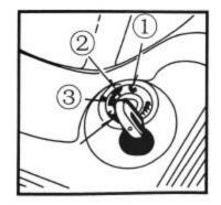
③ LOCK position Turn the switch all the way to the left, push it down and turn it to the LOCK position; the key can be pulled out. In this case, the vehicle can not be steered and the engine as well as the lighting system will not work.
