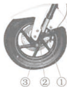
Fig. 31 ① Lock screw ② Speedometer cable ③ Fr. axle nut
