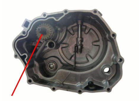
WATER PUMP GEAR
