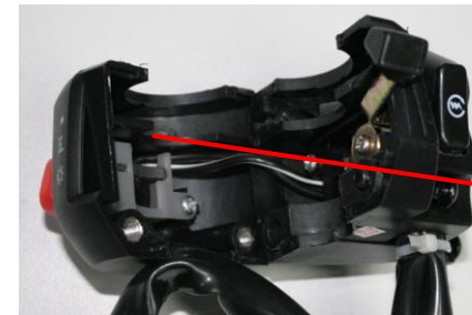
INTERIOR VIEW OF RIGHT HANDLE BAR SW.
