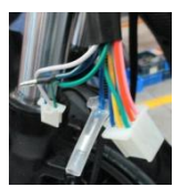
COUPLER OF LEFT HANDLE BAR SW., FRONT LEFT WINKER, METER TO MAIN CABLE
