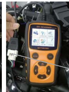
The connecting line is connected with the diagnostic interface on the electronic injection wiring harness.
