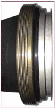
Putting on the sealing o-ring into the slot. The type and measurements are stated in the section: d'Instructions for use "Part I.: Description\_maintenance\_service\_solving problems".
