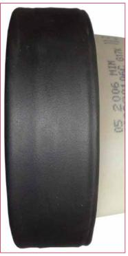
Putting on the fixing o-ring. The type and measurements are stated in the: d'Instructions for use – Part I.: Description\_maintenance\_service\_solving problems. A larger strength is required to put on the o-ring and it is necessary that you check for any folds which cause bad sealing of the system. More information can be found in the section: Instructions for use – Part I.
