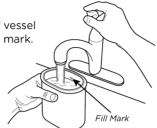
2. Assemble the mold halves and slowly lower into the water. The water should fill above the top holes in the mold - if not, add a little more.
