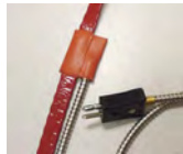
PROCESS SENSOR LOCATED BESIDE THE ELEMENT
