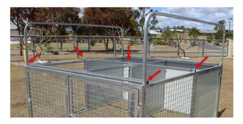
Recheck diagonal measurements are still equal. If they are not, adjust until unit is square. Then tighten all bolts firmly.
