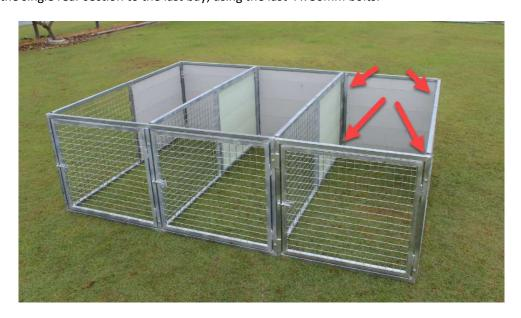
**Step 4.**Measure the diagonal corners of the unit, adjusting until the measurements are the same and the fra
