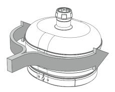
... The flue is designed to have a rain guard which has a 5mm gap from the Dome S1.
