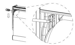
Insert the back edge of the raceway into the back plastic part of the bracket, and then turn the raceway upwards so that the front rib of the raceway snaps into the bracket.
