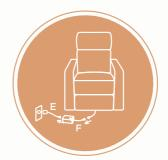
Plug in the two components of the power cord (part E and F), and connect to the back of the chair. Plug into a wall outlet.
