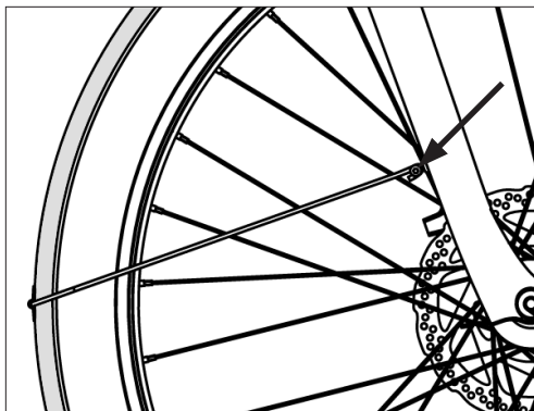
Fig. 22: Mounting bolt on fork lower
