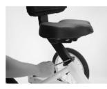
Step 7. Install the assist steering rod and tighten the QR.
