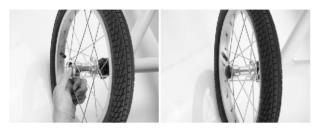
Step 3. Install the front wheel. Insert the threaded axle through the hub and tighten it with 6mm hex wrench. (Torque 6-8nm)
