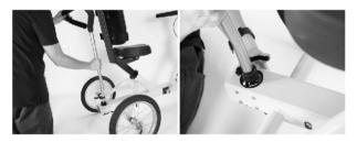
Step 8. Use 15mm open wrench to install pedals (right: clockwise, left: counterclockwise).
