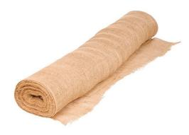
**Product Specification** – Plain weave Hessian Cloth width 1.37m x 46m x 200gms/m2 made of 100% lignocellulosic natural and biodegradable jute fibres .
