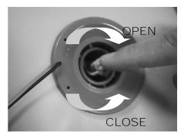
To lock open valve, depress the stem and rotate ¼ turn clockwise. To close valve, depress the stem and rotate ¼ turn counter-clockwise. The valve stem should be in the depressed position while inflating. Replace the cap on valve after inflation to ensure air tight seal.
