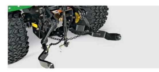
**Rear 3-point Hitch:** Easily hook up and lift heavy rear attachments with the optional 3-point hitch. Optional rear PTO sends engine torque to rear attachments such as a power harrow, sprayer or rear spreader.
