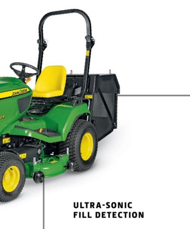
Ever been caught out with a full hopper a long way from the unloading area? The Fill Sensor indicator monitors the real time fill status while you work – and being ultrasonic, it's reliably accurate, too.
