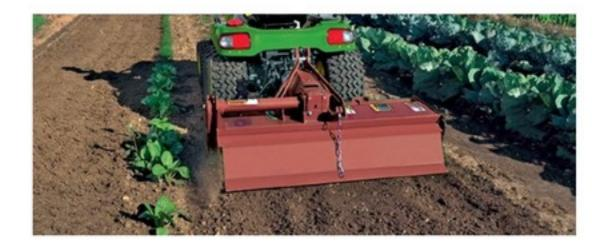
**Rear PTO:** To deliver ample torque for rear implements, add a rear power take off.
