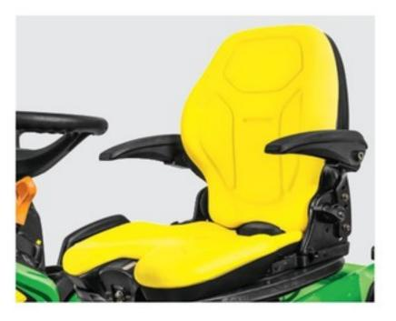
**Seat:** Choose either the comfort seat with adjustable back and optional armrests, or the new air-ride seat with full pneumatic suspension.
