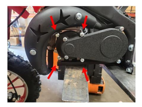
Step 2, Remove the 10mm bolt holding the clutch in place, this is a lot easier with a impact gun than by hand. If you don't have a impact gun this can be done by locking the clutch in place with a flat head screw driver by sliding it through the clutch and wedging it on the engine case. We strongly advise you to use a impact gun of some kind to stop any damage to the cases.
