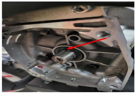
Step 5, put the 10mm bolt back in and tighten it up, push the transfer box back over and tighten the 4 8mm bolts back up
