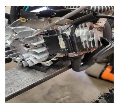
Step 3, Remove the two Allen key bolts holding the coil pack in place
