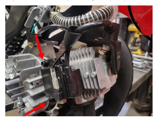
Step 4, Unplug the wire connected to the coil pack as this will save unplugging any wire tucked away in the bike or quad.
