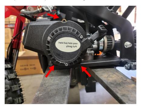
Step 2, Remove the cap from the top of the spark plug
