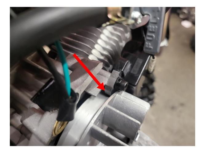
Step 7, Place the pull start back over the engine case ensure the pull start lines up with the fly wheel and tighten the 3 bolts.
