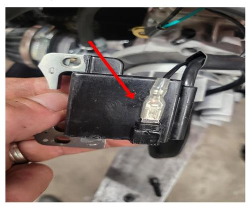
Step 5, plug the wire you just removed from the old coil pack in to the new one and bolt the new coil pack back in place. Do not tighten these two Allen key bolts just yet.
