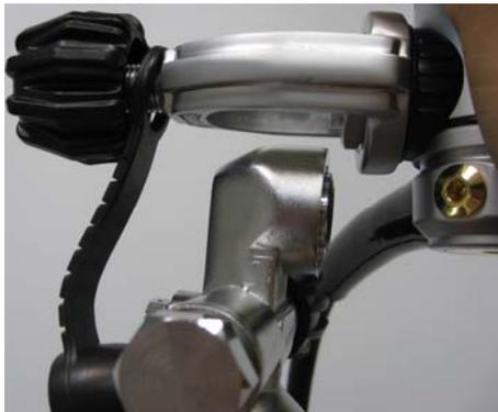
For DIN connector: Remove the dust cap and align the first stage inlet with the tank valve opening. Turn the hand wheel clockwise until snug.
