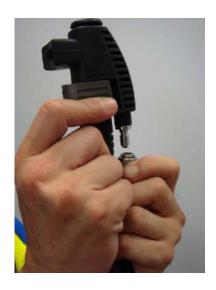
4) Open the tank valve SLOWLY. Check for any air leakage and proper power inflator function before using the BCD.
