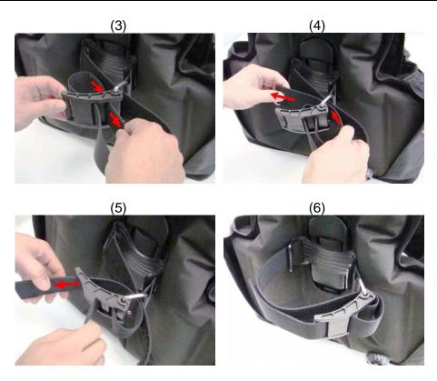
Attaching the BCD to the tank
