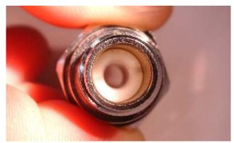
14. To adjust the 2<sup>nd</sup> stage's air output, it can be achieved by either of the following methods: a) with the side plug (part 1) removed, use the 6mm socket to tighten / loosen the nut (part 11); b) tighten / loosen the orifice (part 8) in the orifice seat screw (part 10 – as shown) to increase or relax the lever tension. The later method (b) is the preferred method as it is easier to fine tune.
