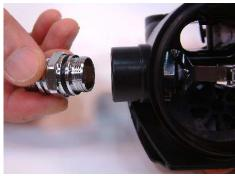
4. Use the adjustable spanner to loosen and remove the orifice seat screw (part 10).
