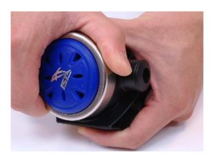
2. To remove, firstly, rotate counter-clock wise to remove the metal bezel (part 18) and purge cover (part 19).
