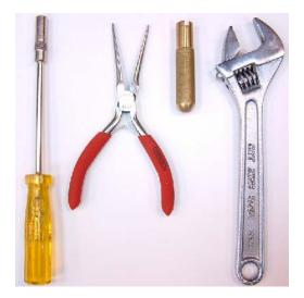
1. The tools shown above are the ones needed to perform the servicing operation of the O40 2<sup>nd</sup> stage / octopus: 6mm socket (with screw driver type handle), a pair of pliers, 4-slot 2<sup>nd</sup> stage tool and an adjustable spanner. If a certain tool(s) is difficult to obtain, appropriate improvisation can be considered, as long as there is no extraneous / unusual stress to cause damage to the 2<sup>nd</sup> stage.
