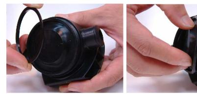
3. Remove the diaphragm washer (part 17) and then the diaphragm (part 16).
