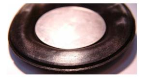
15. The groove around the inside of the diaphragm (part 16) must sit perfectly on the lip of the main housing (part 3) to create a strong seal
