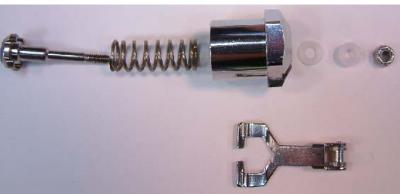
7. To dismantle the lever and valve assembly for servicing, use the 4 notch 2<sup>nd</sup> stage tool to hold the bottom of the poppet (part 5) and the 6mm socket to unscrew the nut (part 11). Be careful not to lose any part when the nut is coming undone as the spring (part 4) will exerts force to restore its original shape.
