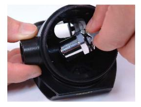
5. Take the lever and brass valve housing (containing part 4~6, 11~15) out of the main housing (part 3)
