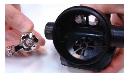
13. When assembling the lever / valve unit, the lever (part 13) should point away from those 2 smaller holes in the brass valve housing (part 15) and the exhaust valve.
