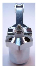
6. Count the number of threads of the poppet (part 5) that is exposed and use this information for reassembling.
