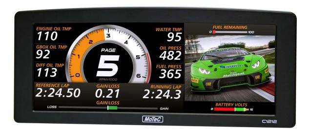
The C1212 comes standard as a combined 12" full colour display and powerful control device with outstanding readability in direct sunlight.
