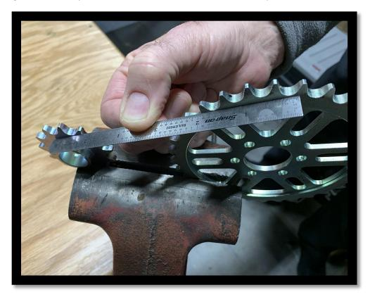
If the alignment gap at the front sprocket is off by more than 1mm, add or remove the shim to bring it back into alignment. Some bikes using the 420 kit will require the alignment shim and some will not. The 219 kit seems to not need it for two reasons: 1) We designed it in house to fit without the use of a shim
