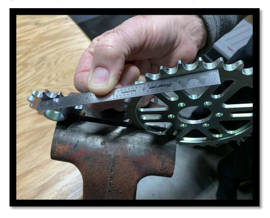
If the alignment gap at the front sprocket is off by more than 1mm, add or remove the shim to bring it back into alignment. Some bikes using the 420 kit will require the alignment shim and some will not. The 219 kit seem to not need it for two reasons: 1) We designed it in house to fit without the use of a shim and 2) Due to many more links the 219 will accept more misalignment without the excessive noise and wear. Always check the alignment when installing your kit.
