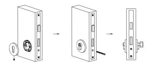
7.Attach the escutcheon to the inner rose, use the  $\phi 2$  Allen Wrench to fasten the M4x6 Allen screws, then install the cylinder screws.
