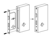
2.Install the mortise with the wood screws.
