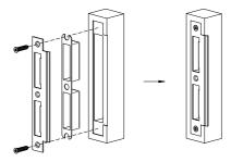
8. Place the striker plate on the door jamp ensuring it is correctly located relative to the mortise. Mark this position, then chisel and drill out the striker cutout.
