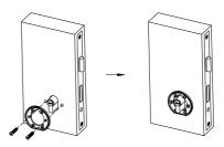
6.On one side, install the inner rose, adjust the position and stabilize with the M4x28 connecting screws.
