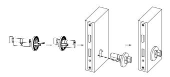
5.Insert the escutcheon through the cylinder, then insert the cylinder to the mortise.
