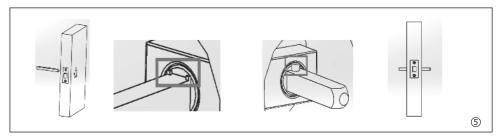
⑤.For the PRIVACY handles function, press down the button on the spindle and insert the spindle though the latch so the spindle cannot be pulled out For PASSAGE handles, there are 2 spindles. Insert one of them (depending on your door thickness) through the latch, and adjust the position according to the thickness of the door.
