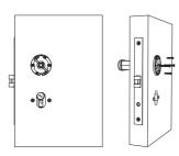
6.Install the right side's mounting kit and locating piece, adjust the position and stabilize with connecting screws and wood screws.
