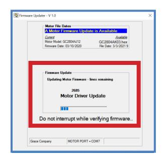
You will now be prompted to **POWER CYCLE the motor carriage then turn the sewing machine back ON**. Turn off
