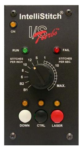
a warning light. If it flashes when you are using regulated stitching mode, it is indicating that the stitches have reached twice the chosen length and you are moving the machine too fast. It will be continuously lit when the controller detects a needle jam.
