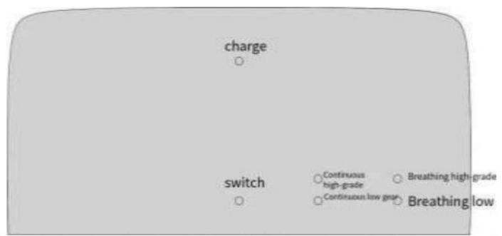
When charging, the "charging" indicator light is on. When charging is completed or not, the "Charging" indicator goes out.
