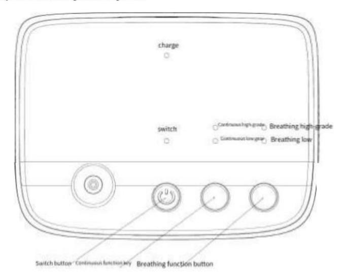
Press the "switch" button in the power-off state, and the "switch" indicator light will be on, and the machine will enter the power-on state. Press the "switch" button in the power-on state, the "switch" indicator goes out and the machine is turned off.
