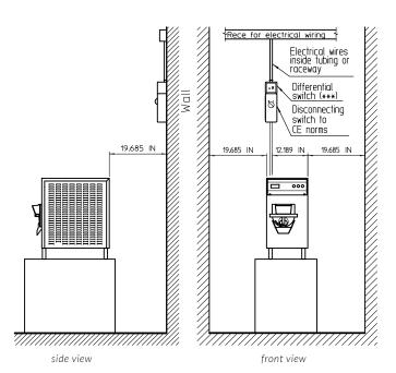
(\*) even if the machine models vary, the water and electricity connection positions are always the same, i.e. on the LEFT side of the machine.
