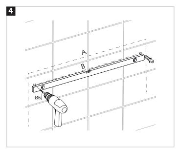
Drill the marks using an 8mm drill bit and ensuring there are no hidden pipes or cables in the wall. Make sure the correct drill bit is used for the surface being drilled and check that the holes are level.
