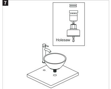
Prepare worktop for taps and basin waste. Cut holes where required using a suitable sized "holesaw' at a slow speed.
