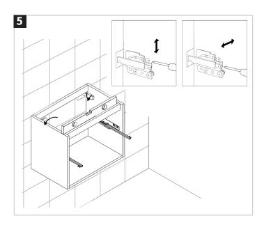
Install the wall brackets using the fixings provided. The unit carcass can now be mounted on the wall brackets and adjusted to ensure it is flush with the wall and level.
