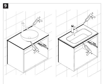
Apply silicone sealant to the joins between the basin and unit on all sides to keep watertight. Check the manufacturer's instructions for drying times.
