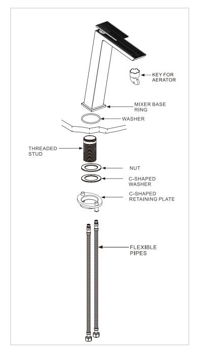
Screw the flexible pipes into the mixer body, and fully hand tighten. Place mixer in position to see if any alteration to the existing supply pipework is necessary. After making any necessary alterations to the pipework, pass the mixer base ring and washer over the flexible pipes and threaded stud to form a seal on sink top. Pass the tails and fixing stud through the hole in the basin from above and place the mixer in position on the basin.
