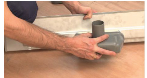
Place outlet onto the main drain body and clip into position. Attach push fit adapter into the outlet.
