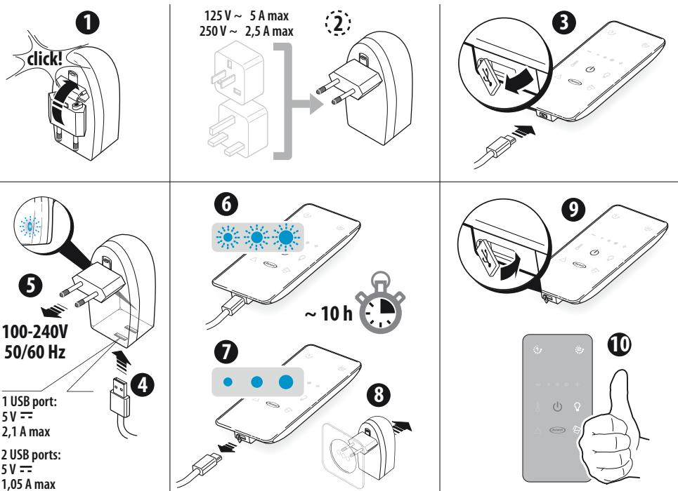
■ Once charging is complete, reposition the USB cover (fig.9). Where not used, disconnect the battery charger from the socket.
