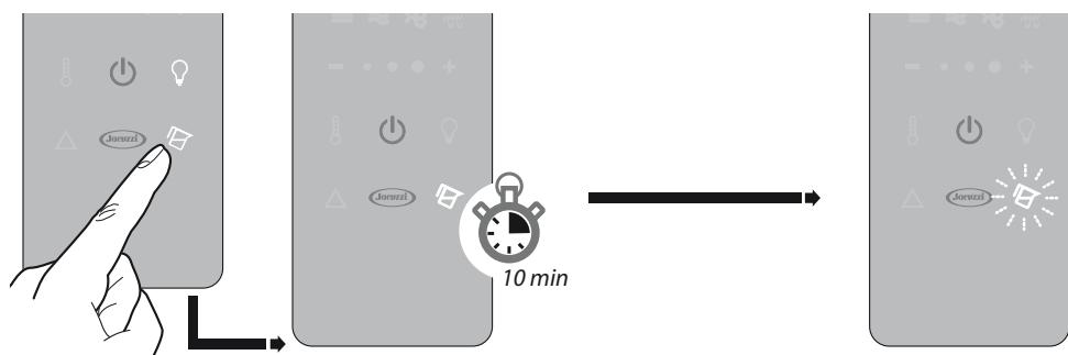
The function lasts approximately 10 minutes and is completely automatic; about one minute before the end of the function, the pump activates once again to rinse the pipes.
