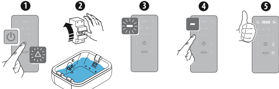
■ If the "--" key flashes, keep it pressed down until the symbols denoting the various functions light up (fig.5): the remote control is now ready.
