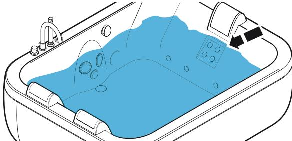
■ Check that the outlet nozzles along the tub perimeter are open.
