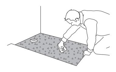
6) Remove the protective cover. Apply cement-based single part flexible tile adhesive to the entire underside of the shower board.
