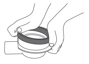
2) Place the retaining ring with seal ring on the floor drain and push it down firmly until it audibly clicks into place.
