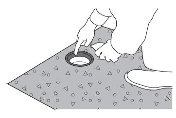
8) Position JACKOBOARD® Aqua Line easy in the screed recess, making sure the drain nozzle on the channel fits into the seal ring on the drain.
