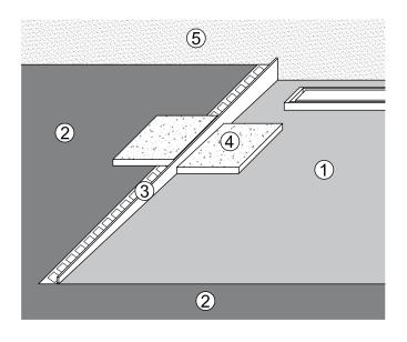
For shower elements with a fall on one side, the side edge to the screed can be covered with the fall profile JACKOBOARD® Aqua Line Profile (available as an accessory). The sloping profile is available as a left version (illustrated) or as a right version.
