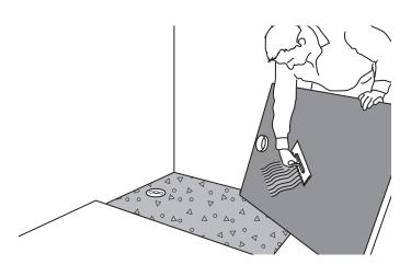
7) Grease the seal ring on the floor drain to facilitate installation of the shower board.
