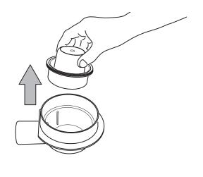
1) If the floor drain contains an odour trap, it must be completely removed (top and bottom sections). The shower drain channel is already fitted with a special odour trap.
