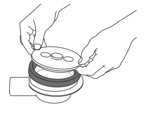
3) Cover the floor drain with the protective cover.
