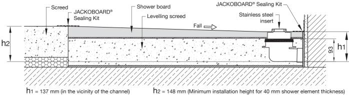
112 = 146 min (withinfilm installation neight for 40 158 mm (Minimum installation height for 50
