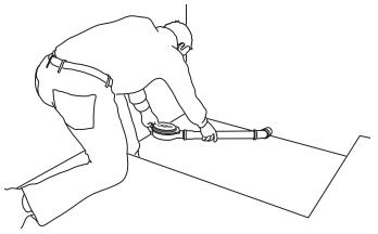
4) Insert the floor drain into the existing DN 50 pipe. Make sure the drain is at the right height and position (see the illustration "Installation height", Pages 6 and 7).
