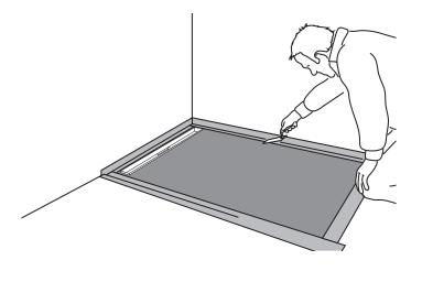
9) All connecting joints are sealed with the JACKO-BOARD® sealing set (or equivalent).
