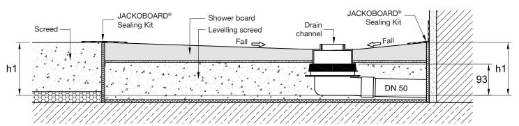
h1 = 148 mm (Minimum installation height for 40 mm shower element thickness) 158 mm (Minimum installation height for 50 mm shower element thickness) 168 mm (Minimum installation height for 60 mm shower element thickness) 178 mm (Minimum installation height for 70 mm shower element thickness)
