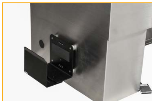
OA-145 - CPU WALL MOUNT Designed to fit CPU's from 4, 6, and 8 in. wide. Units are constructed from heavy duty aluminum, with neoprene padding to protect your CPU as it is clamped securely into the mount.
