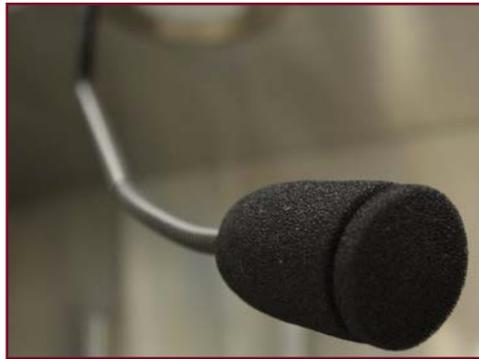
**OA-109 - MICROPHONE ON FLEX ARM** Easy-to-adjust, small-diameter, alternating gooseneck provides a steep low frequency attenuation to improve sound pickup without affecting voice quality.
